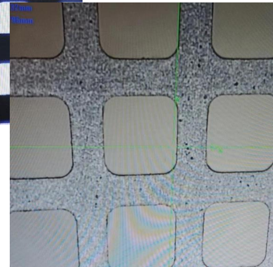
Hole Diameter: 0.1*0.1mm 50x Magnified Effect
