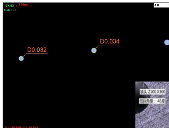
Hole Diameter: 0.035mm 300x Magnified Effect
